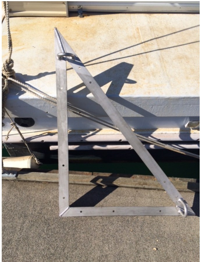
CNC Waterjet cut Corner brackets & Pole Guides
